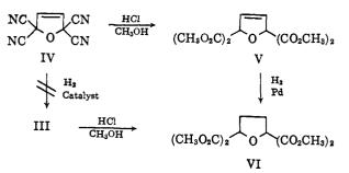
It has not yet been possible to reduce IV to III catalytically, but IV has been converted to the corresponding tetraester V,<sup>4</sup> m.p. 96.5–97°. Catalytic reduction of V gives the saturated ester VI,<sup>4</sup> m.p. 103–104°, which is identical with that synthesized from III.
