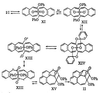
$(180^{\circ})$  about the bond joining the two halves of the dimer gives XV which collapses to II. III may be produced by thermal rearrangement of dimer II molecules formed in a vibrationally excited state or by a separate photochemical process.<sup>8</sup>
